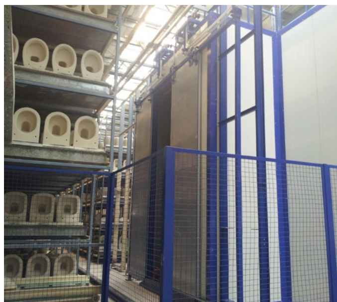
干燥机出口及产品储存 Dryer exit and product storage
