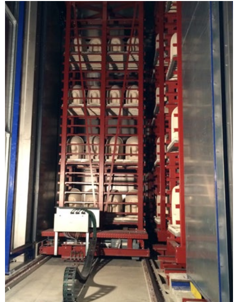
干燥机出口的干燥车摆渡车 Dryer exit transfer car with dryer car
