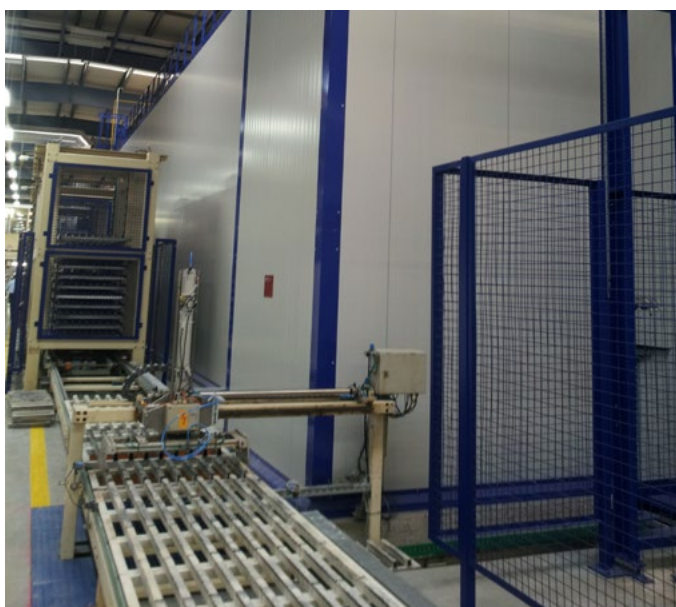
有托盘回转输送线的干燥机入口 Dryer entrance with pallet return conveyer
