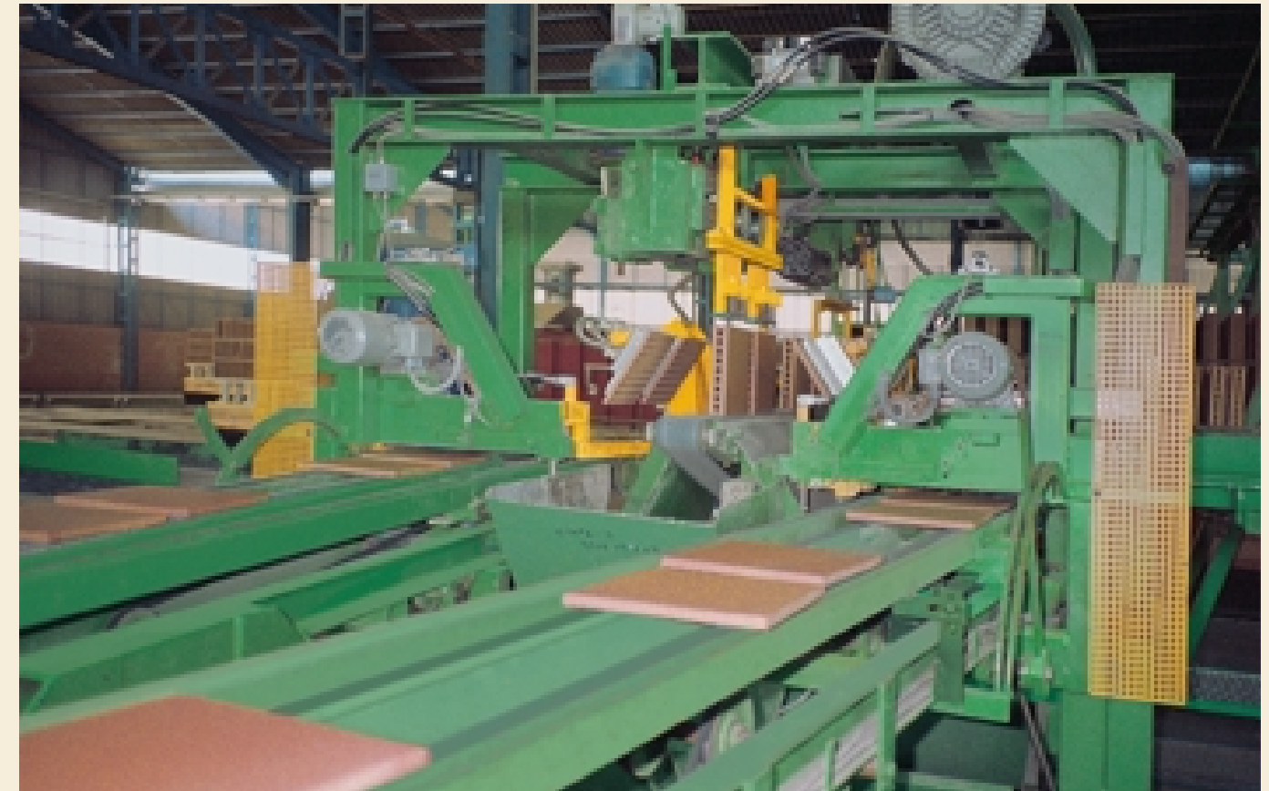
▼ Tile splitting unit for vertical splitting and setting down with the visible surfaces upwards
