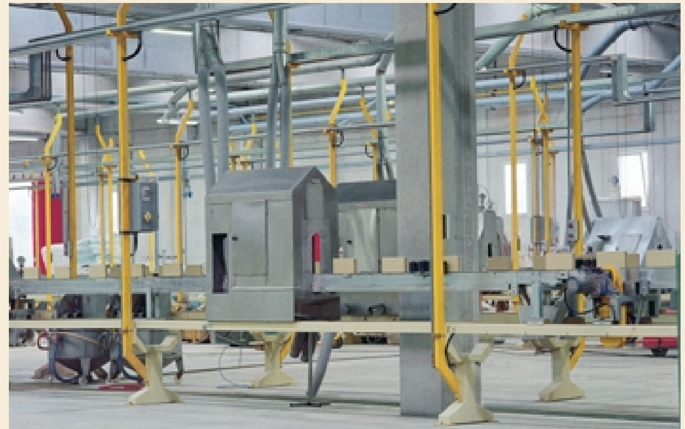
▼ Multi-line glazing stations for two-sided dry glazing using the Lingl centrifugal process for high-quality glazes, also with special colour effects and different coating layers. In combination with compressed air spray systems and special drives, specific shading effects can be produced and even the most demanding glazing requirements met.
