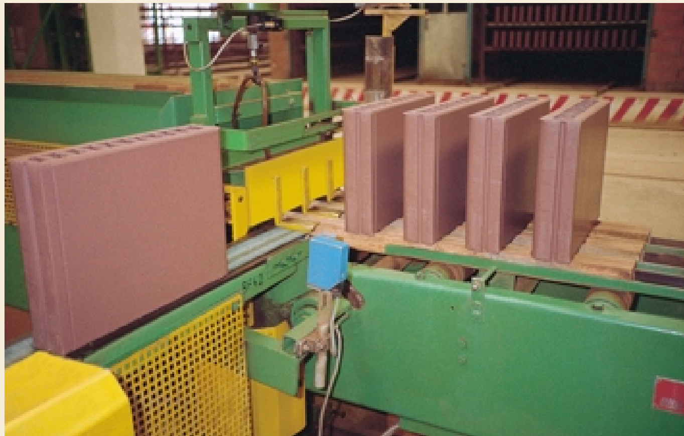
▼ Stairway step double tiles are set down on the drying supports.
