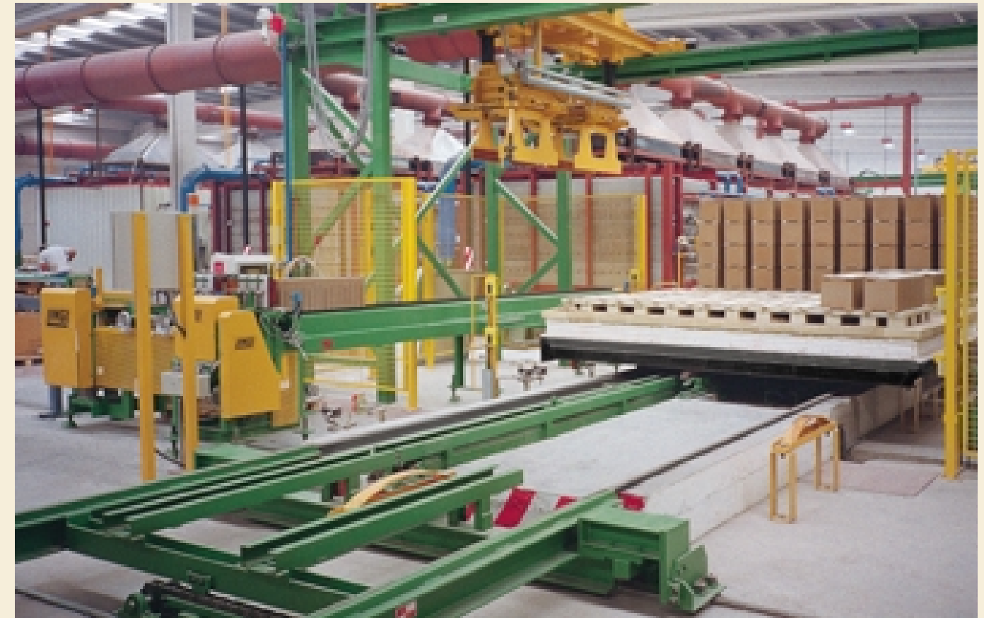
▲ Split tiles are unloaded in rows from the kiln car, separated and passed to the splitting unit
