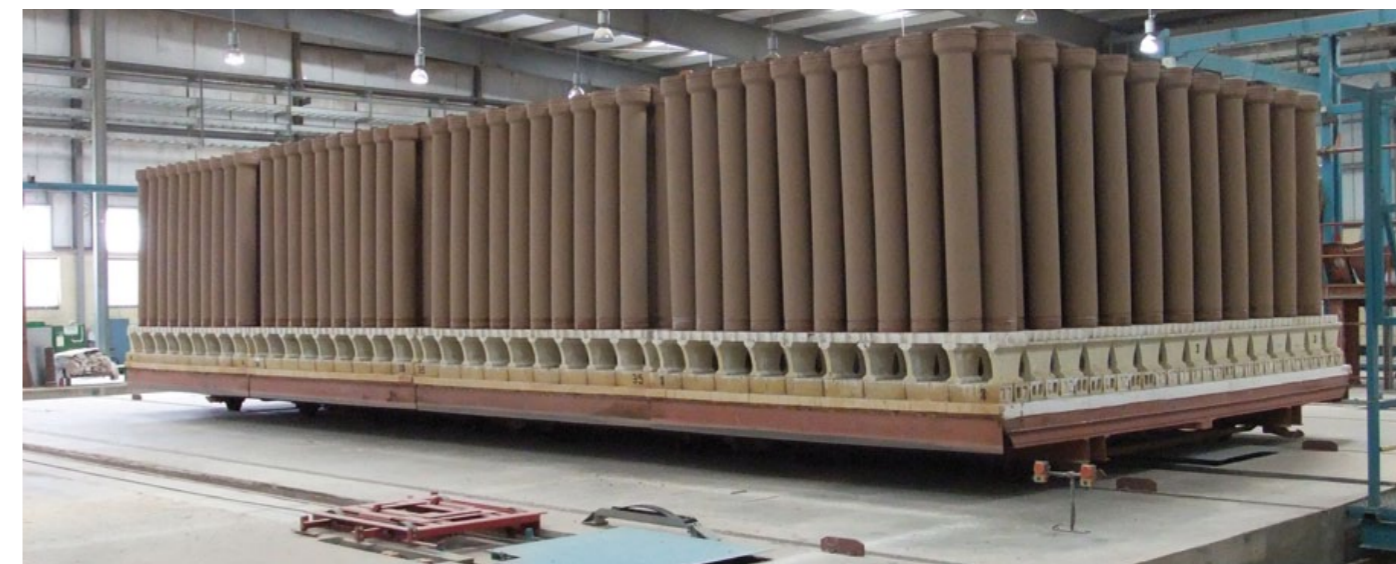
Tunnel kiln car with vitrified clay pipes Wagons du four tunnel chargés de tuyaux en grès
